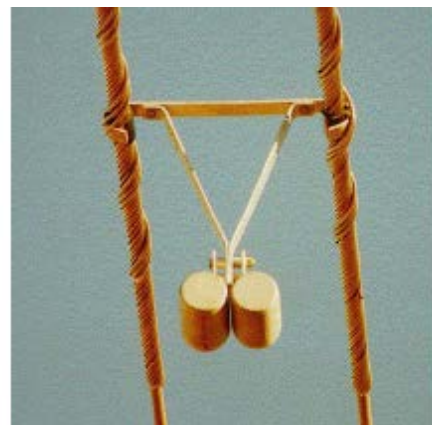
Fig. 5. Detuning Pendulum installed on the twin bundle
