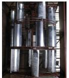
The simple design of wind installation with the vertical rotation axis turbine which includes a base part consists from four ferro-concrete poles located in corners of a square with distance in light between them of 2.8 m. The turbine base part represents frame with the girders, established on top of poles. The frame with the turbine is fixed on horizontal girders. Turbine levels are turned in space rather each other on a corner in 15°.
