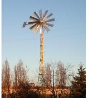
Modernization of wind turbine by increase in its diameter, rotating head for free orientation of wind turbine in wind direction and change of moment transfer direction from a horizontal plane in vertical, generator section in structure of planetary reducer and asynchronous generator is executed. The control and protection system of an electric part of installation is improved.
