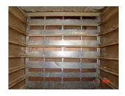
Drying the chamber represents a number of lattices divided by screens which provide stream passage of drying air in a cross-section direction of layer. Air intake is carried out separately for each lattice.
